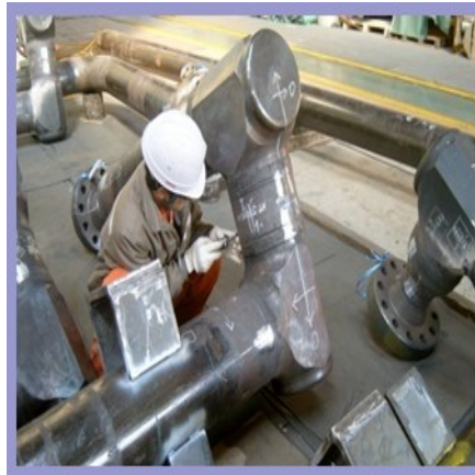
11. H/D (Hardness Test)
