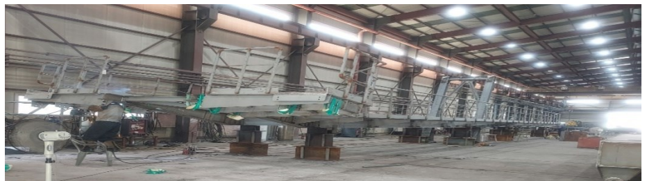
ST/RE _ TRIPPER FRAME
