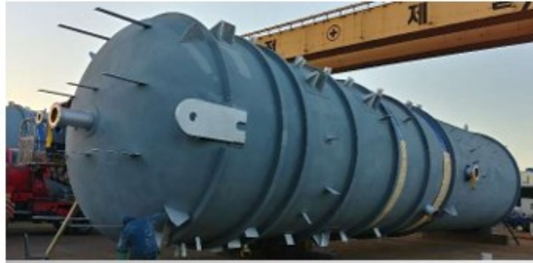
Hot Oil Surge Drum for Hyundai Oil Bank
