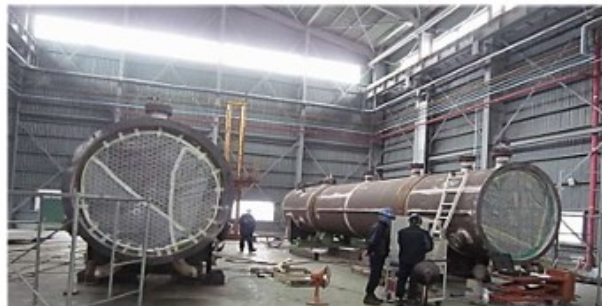
Reboiler Exchanger (USA)
