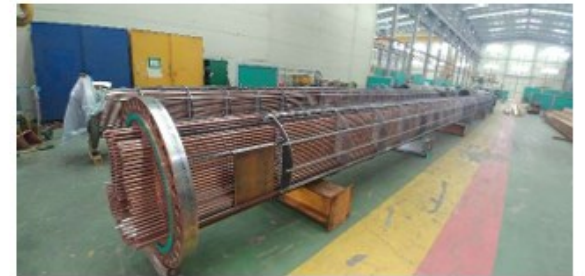
CuMn2 Heat Exchanger (LG IPA)
